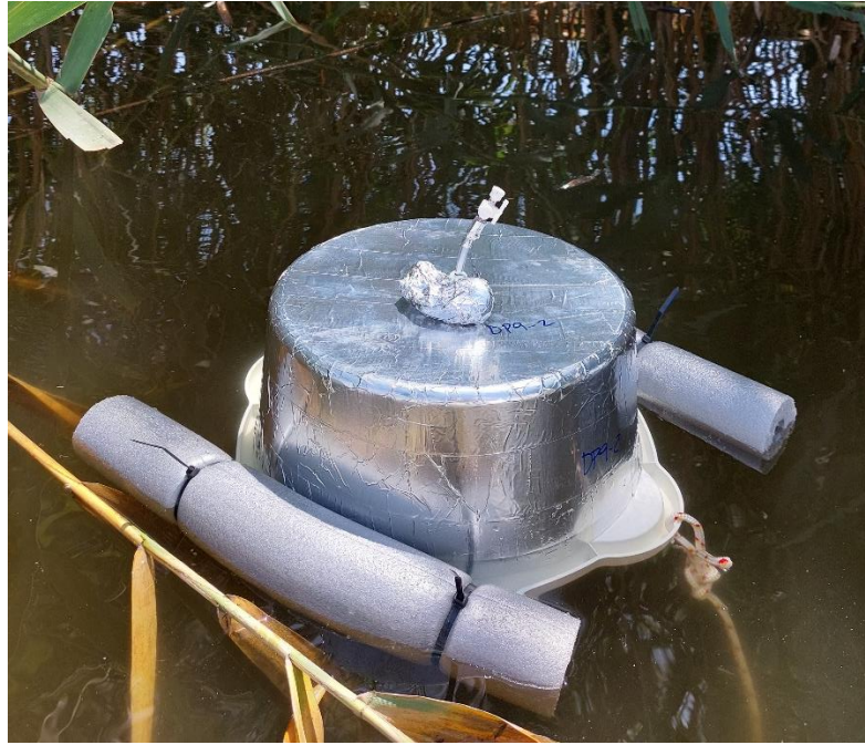
Figure 2: Photo of a gas chamber which is used to collect GHG emitted from ponds. Gas chamber design belonging to Thomas A. Davidson, (2020).
